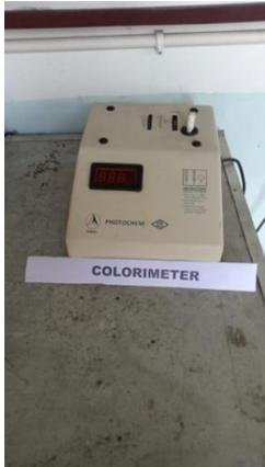
A **colorimeter** may be used to measure the concentration of a chemical in a solution if the chemical imparts a characteristic colour to the solution.
