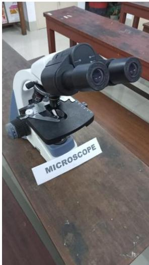
A **microscope** is an instrument that is used to magnify small objects. Some microscopes can even be used to observe an object at the cellular level, allowing scientists to see the shape of a cell, its nucleus, mitochondria, and other organelles.
