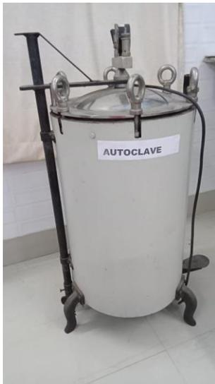
**Autoclaves** provide a physical method for disinfection and sterilization. They work with a combination of steam, pressure and time. Autoclaves operate at high temperature and pressure in order to kill microorganisms and spores.
