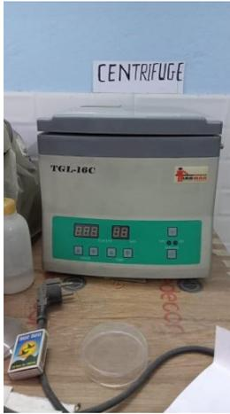
A **centrifuge** is a device that uses centrifugal force to subject a specimen to a specified constant force, for example to separate various components of a fluid. This is achieved by spinning the fluid at high speed within a container, thereby separating fluids of different densities (e.g. cream from milk) or liquids from solids.
