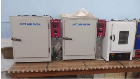
**Hot air oven** is a type of heat sterilization equipment used in various laboratories. This amazing testing instrument will easily destroy the microorganisms as well as bacterial spores with precise temperature control.
