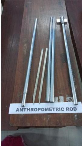
An **anthropometric rod** is an instrument that as its name indicates ("anthropos" suffix from the Greek and indicates "relative to human body", and "meter" that means "measure") is used to measure widths and lengths of bones of human body depending of its range.
