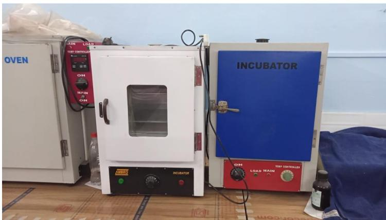
An **incubator** is a device used to grow and maintain microbiological cultures or cell cultures. The incubator maintains optimal temperature, humidity and other conditions such as the CO<sub>2</sub> and oxygen content of the atmosphere inside.
