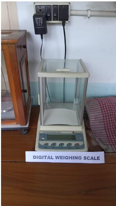
**Digital weighing scales** are devices used to measure the weight or mass of an object. They are sometimes called electronic scales and are usually composed of an LCD screen, load cell, controller and platform.
